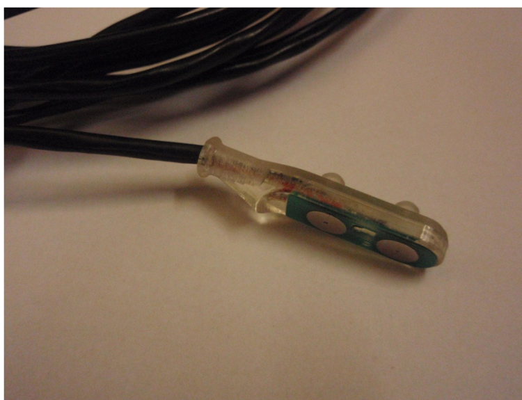
Figure 1 Non-polarizing MR compatible electrode with an eight meter twisted pair cable used for recording skin conductance levels of subjects while lying in the scanner.
